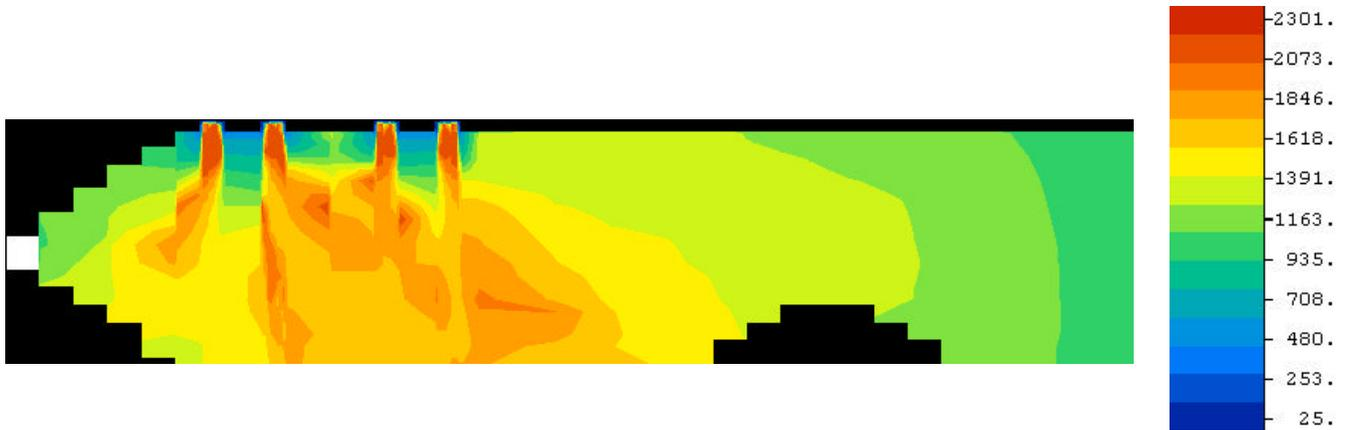
**Fig.3 a - Temperature Contours of a Full scale power station boiler**
